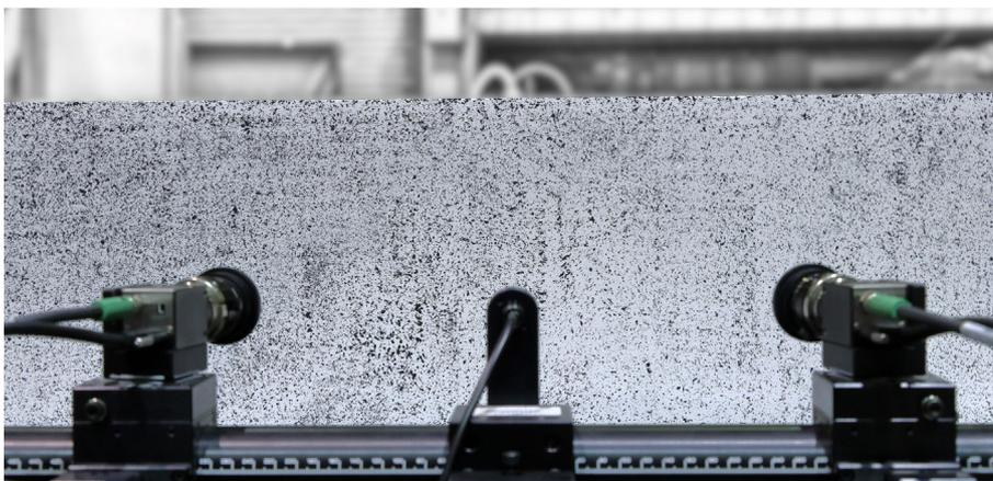
FIGURE 11 Speckle Pattern and Cameras for DIC Strain Measurements
